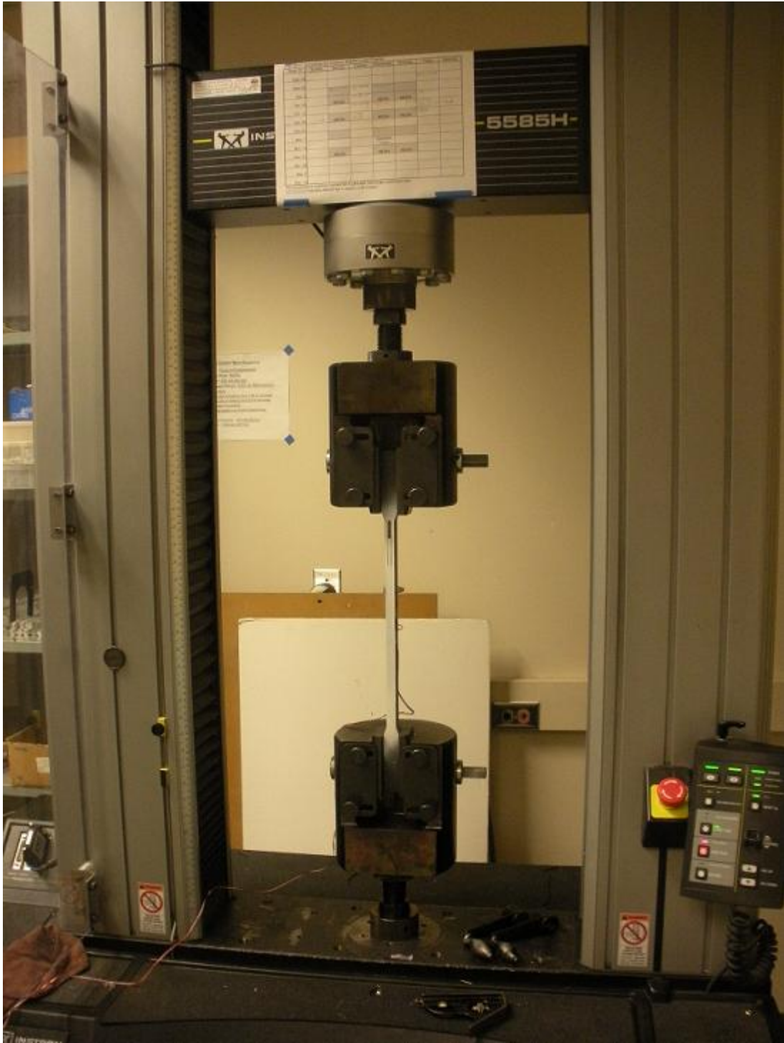
Figure 3.2: Specimen loaded in Instron load frame.
