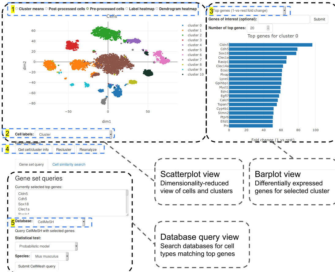
Figure 4.2: This figure shows the main user interface of UNCURL-App. The top left contains the scatterplot, showing a views of the cells and clusters. The top right is a barplot containing the top genes per cluster. Clicking on a cluster in the scatterplot updates the top genes. On the bottom is the database query view, which is used to identify cell types present in the dataset. Options: (1) These are options for what type of visualization to show in the scatterplot. "Cluster means" shows one point for each cluster. "Post-processed cells" shows a dimensionality-reduced view of cells that takes the W matrix returned by UNCURL as input. "Pre-processed cells" (default) shows a similar view, but using the original data as input for dimensionality reduction. "Label heatmap" shows a comparison of two cell label sets. "Dendrogram heatmap" shows a clusters vs genes dendrogram. (2) Options for how to color the cells/points in the scatterplot. Can be based on cluster, gene expression, or a custom label set. (3) Options for how to identify the top genes. Can be 1-vs-rest or pairwise, p-value or ratio. (4) "Get cell/cluster info": get read/gene count for the selected cell and cluster. "Recluster": options to merge, split, delete, or create a new cluster. "Reanalyze": options to re-run the whole analysis. (5) There are a number of databases that can be used for cell type identification, including CellMarker, CellMeSH, and Gene Ontology.
