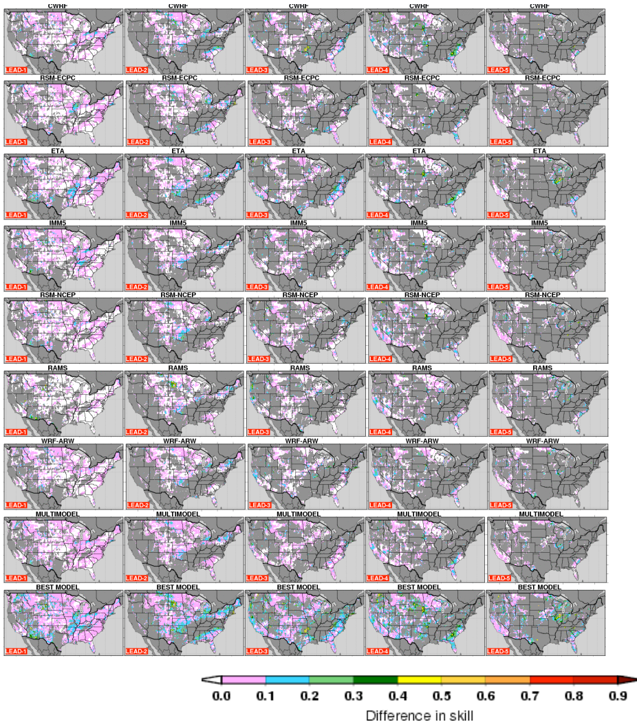
Figure 5.4: The difference in runoff forecast skill derived from dynamically and statistically downscaled CFS forecasts. Each of the first seven rows represent the runoff forecast skill (correlation between ensemble mean forecast and observations) obtained from the RCMs used in the MRED project, individually. The last two rows represent the skill of Multimodel average (Average of all RCMs and all ensembles) and of the RCM
