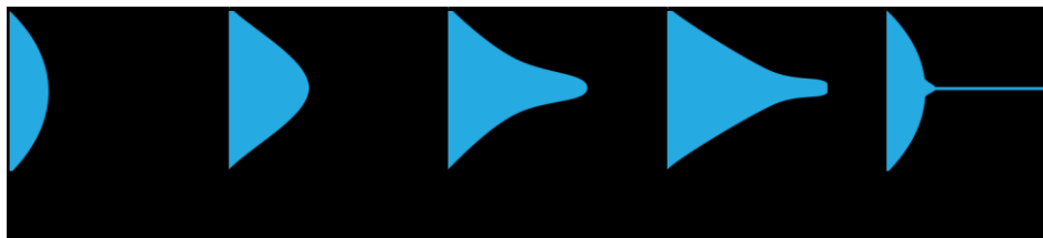
Figure 1. Taylor droplet voltage-geometry history when high voltage applied resulting in a nanofiber stream in far right plate. [32].
