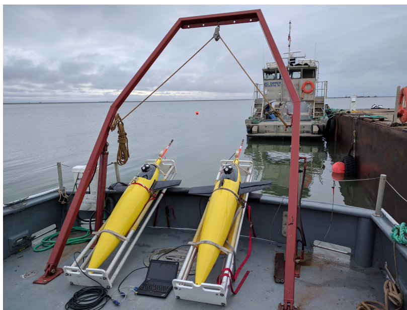
Figure 7.1: Ready for launch, Seagliders SG196 and SG198 are loaded on the R/V Ukpik in Prudhoe Bay, AK, with the upward-facing ADCPs visible where they are installed in the aft fairing.
