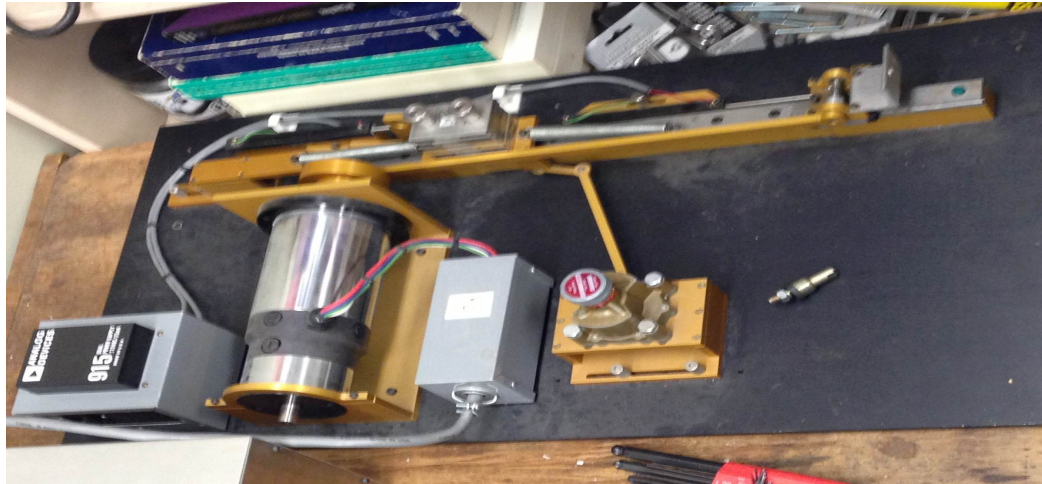
(a) Linear Actuator and Motor Set-up for Dynamic Tests of the Dampers Attached to the Tail/Rudder System
