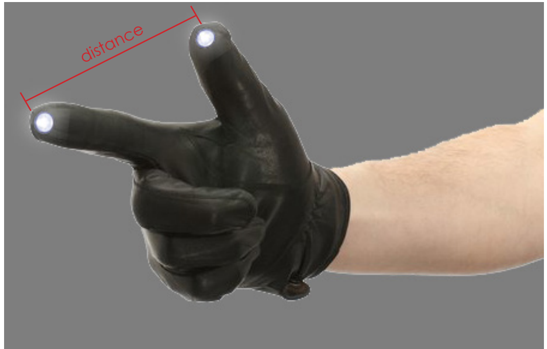
Figure 37: two fingertip LEDs recognition
