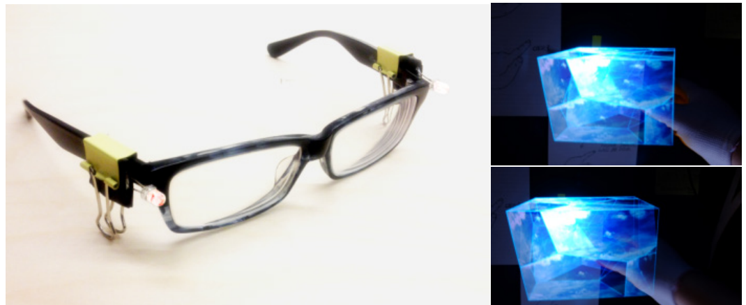
Figure 41: reviewing the same geometry from different angle via head mounted IR LED on my glasses.
