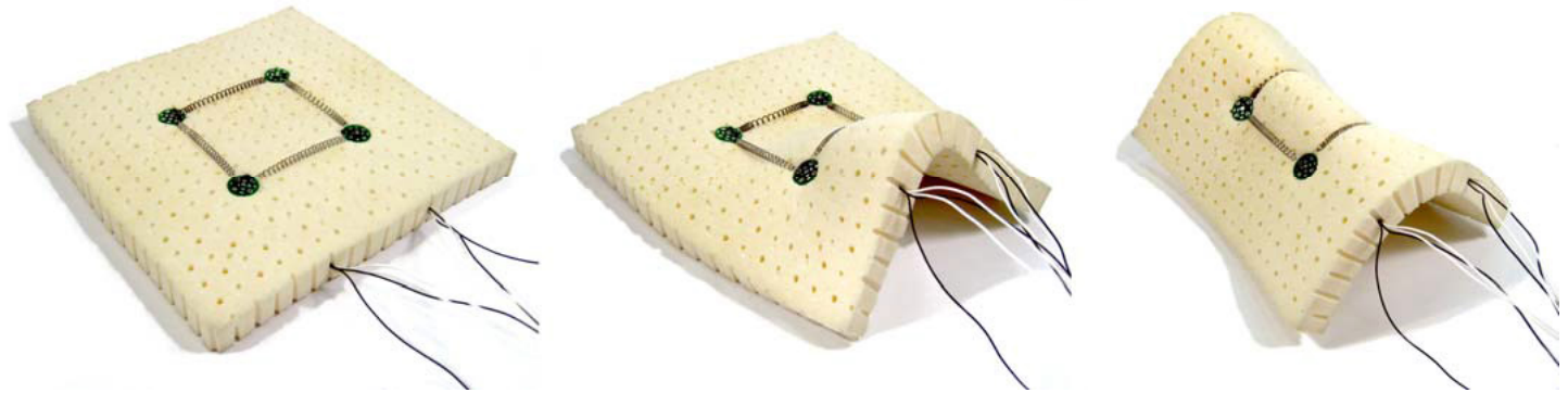
Figure 26: Surfex's surface deformation in three steps
