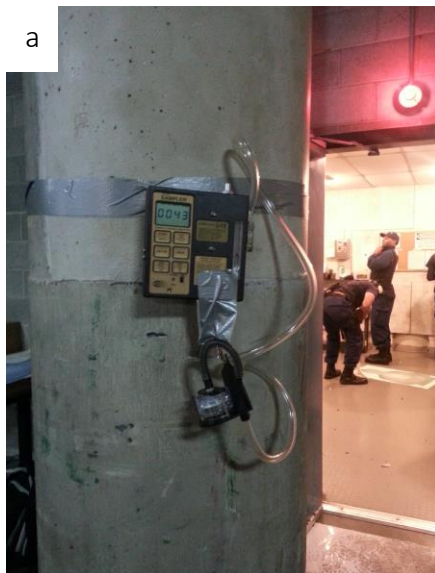
Figure 15a and b Area sampling pumps. On the left, one area sampling pump is located approximately 5 feet from the range's door at a height of 5 feet from the ground. On the right, two area sampling pumps; one placed in firing lane #2 and the other at firing lane #3 (both at a height of 5 feet).
