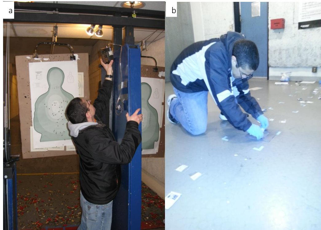
Figure 16a and b UW researcher at work. On the left, researcher setting up area sampling pump at firing lane #2. On the right, researcher taking surface wipe samples from the floor inside the firing range (Photos by MA Torres).
