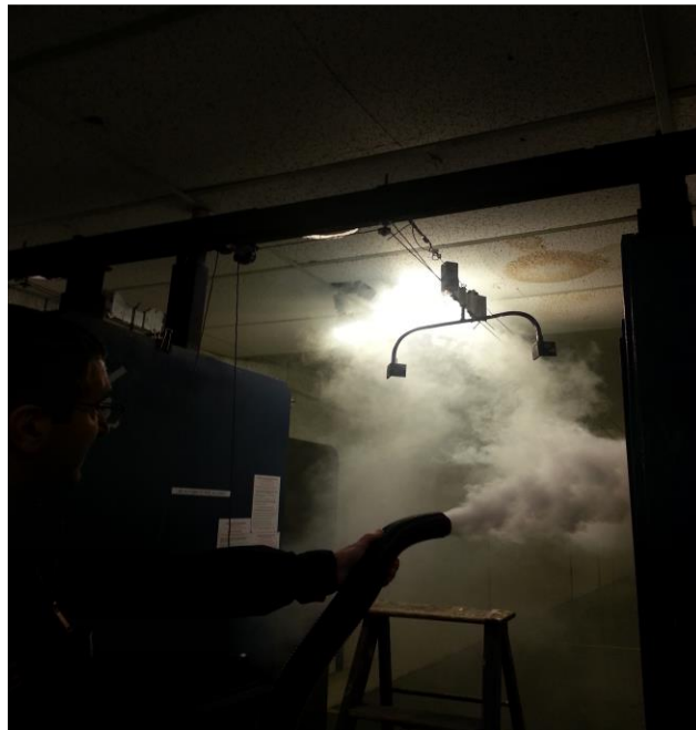
Figure 12 A Rosco® 1500 smoke machine. Smoke was released in all firing lanes simulating each firing positions (prone, kneeling, standing) to observe airflow patterns during normal ventilation operations throughout the firing range (Photos by MA Torres).
