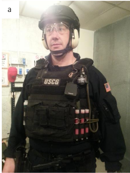
Figures 14a and b FAIs wearing personal air sampling pumps. (a), an MCE filter with a cassette holder is attached with a clip into the FAI's lapel. (b), an FAI has the air sampling pump attached with a clip on his belt.
