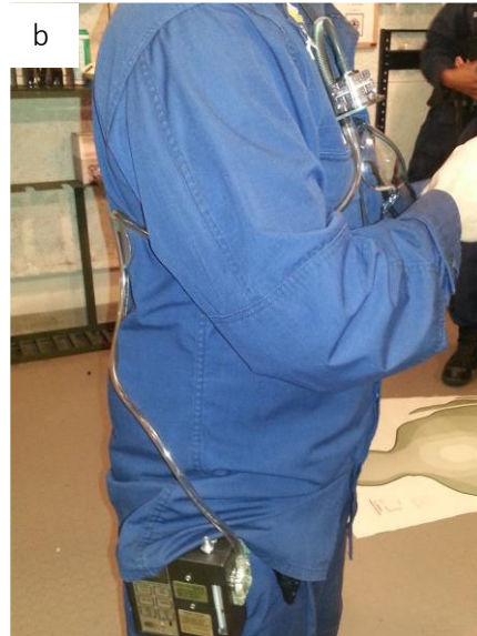
Figures 14a and b FAIs wearing personal air sampling pumps. (a), an MCE filter with a cassette holder is attached with a clip into the FAI's lapel. (b), an FAI has the air sampling pump attached with a clip on his belt.
