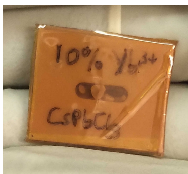
Figure A.2: Photograph of 7.4% Yb 3+ :CsPbCl 3 single-crystal sample sealed in a Teflon mount for air-free EXAFS measurements. The crystal's edge lengths are ca. 1.5 mm. The crystal is centered in the Teflon mount, in the center of the image. CsPbCl 3 and 0.9% Yb 3+ :CsPbCl 3 samples were mounted similarly.
