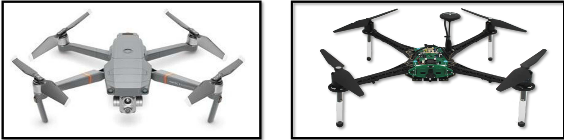
Figure 5.3: Flight Test Hardware. (Left) DJI Mavic 2 Enterprise Advanced; (right) ModalAI m500 Development Drone
