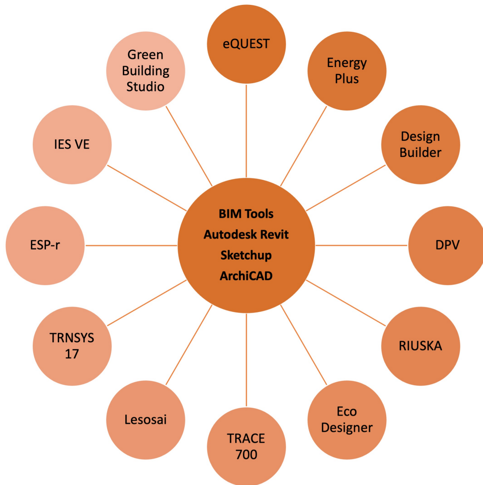
Figure 2.6: The data exchange between the design tools and the energy modelling tools [3]
