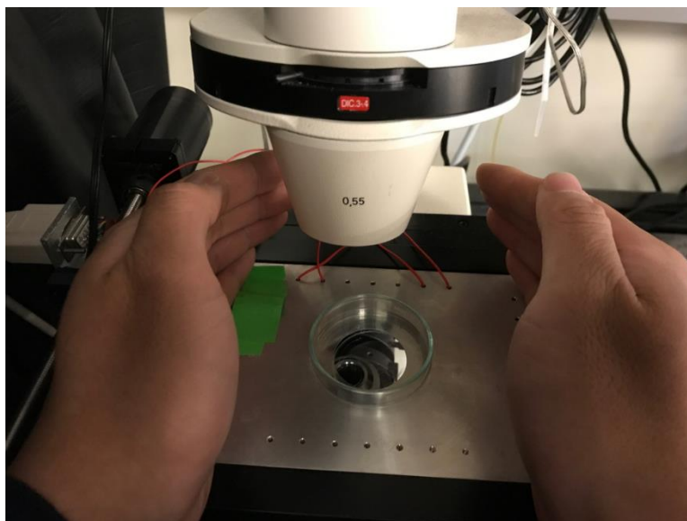
Fig. 3.7. Using hands as an IR source. A demonstration of an experimental configuration.
