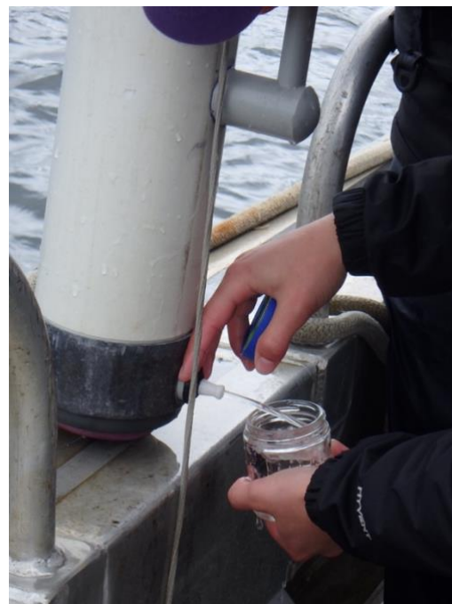
Figure 4. Closing bottle used for taking discrete water samples (photo credit: C. Greengrove).
