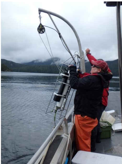
Figure 3. CTD instrument being lowered into the water in for data collection (photo credit: C. Greengrove).
