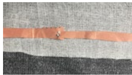
FIG. 18: SOLDERING COPPER FIBER
