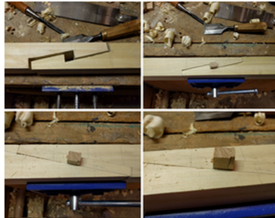
Figure 6.1 - Stop Splayed Oblique Scarf with Through Wedge
