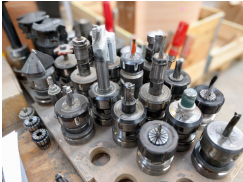
Figure 3.5 – CNC Tool Heads: Various cutting tools for a 5-axis CNC router equipped with an automatic tool changer (Photograph by the Author)
