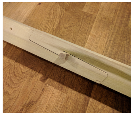
Figure 6.9 – Physical Model - Stop Splayed Scarf. Cut on a 3-axis CNC Router
