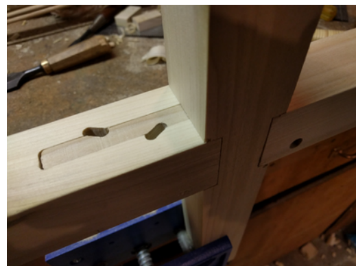
Figure 6.11 – Physical Model – Pinned and Keyed, Shouldered Mortise and Tenon for Post and Beam Connection
