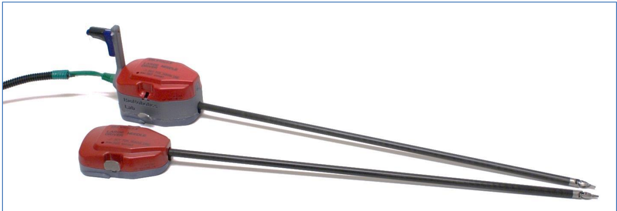
Figure 13 - Retrofitted da Vinci training instrument with sensor housing on back end.
