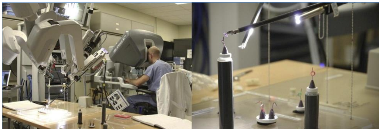
Figure 10 - Experimental set-up. Demonstration of proficiency modules in their respective jigs and the plumb lines draping down onto the jig to ensure standard robotic arm positioning.
