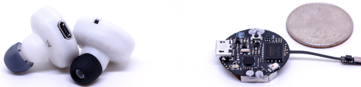
Figure 1.3: An image of the ClearBuds hardware. We built the first binaural headset that could stream time-synchronized audio to a mobile phone.
