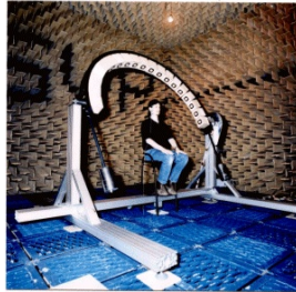
Figure 5.2: Example from Southampton (2003) of an anechoic chamber and speaker array for measuring HRTFs
