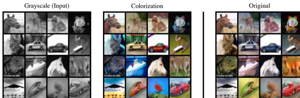
Figure 7.7: Colorizing CIFAR-10 images. Left: original CIFAR-10 images. Middle: greyscale conversions of the images on the left. Right: imputed colors for the greyscale images, found by BASIS using NCSN as a prior.
