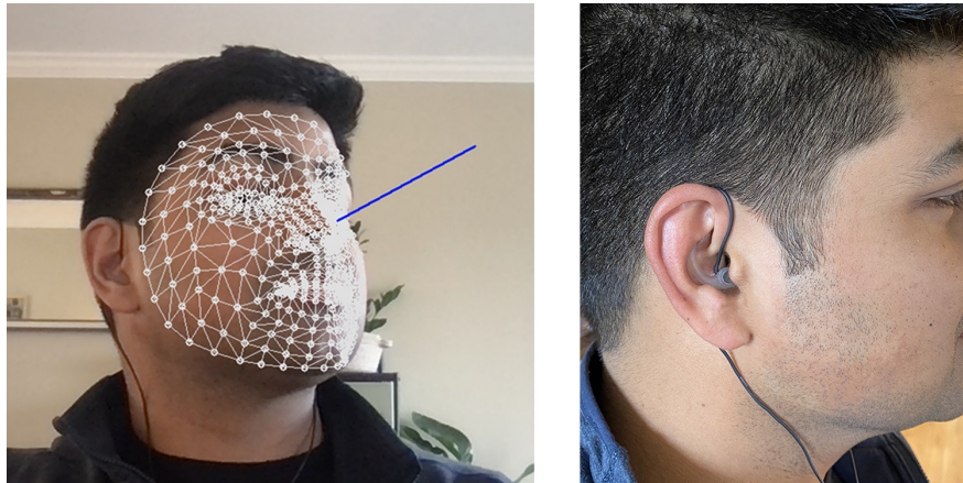
Figure 5.4: Left: Our head tracking implementation uses the webcam to determine the 3DoF head rotation during recording. The normal vector is drawn in blue to help visualize the direction the head is pointing. Right: An image of the binaural microphone used in our implementation. The microphone sits near the ear canal.
