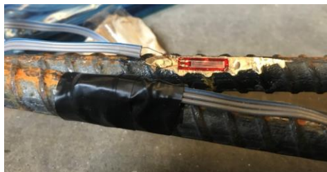
Figure 4.5: Photo of two strain gauges at different stages of installation
