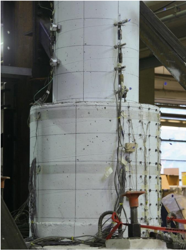
(a) Inclinometers, Duncan potentiometers, and string potentiometers at the column base (north side)
