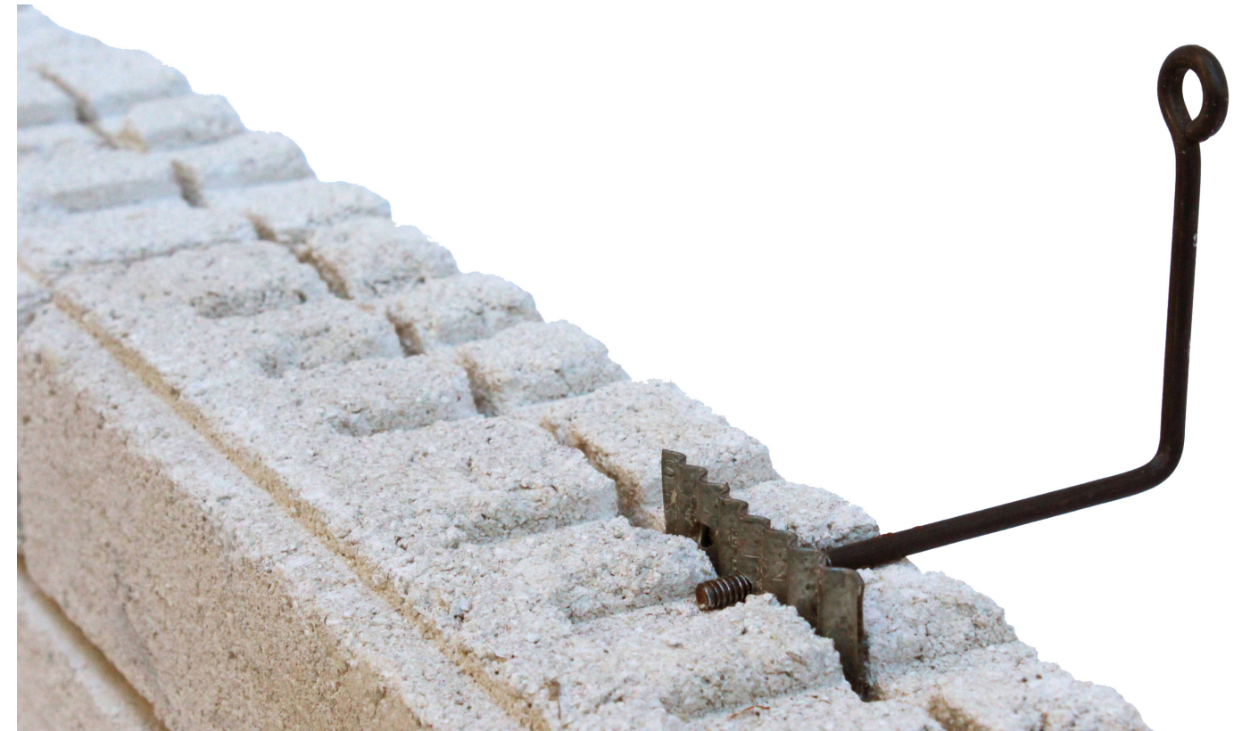
Figure 8.24 Masonry ties are fastened to the bricks through threaded holes in corrugated mechanical fasteners. The fastener location can be adjusted to any of the six indentations in order to align with wall stud locations in the structural backing wall (Photo by Jeremy McGlone)
