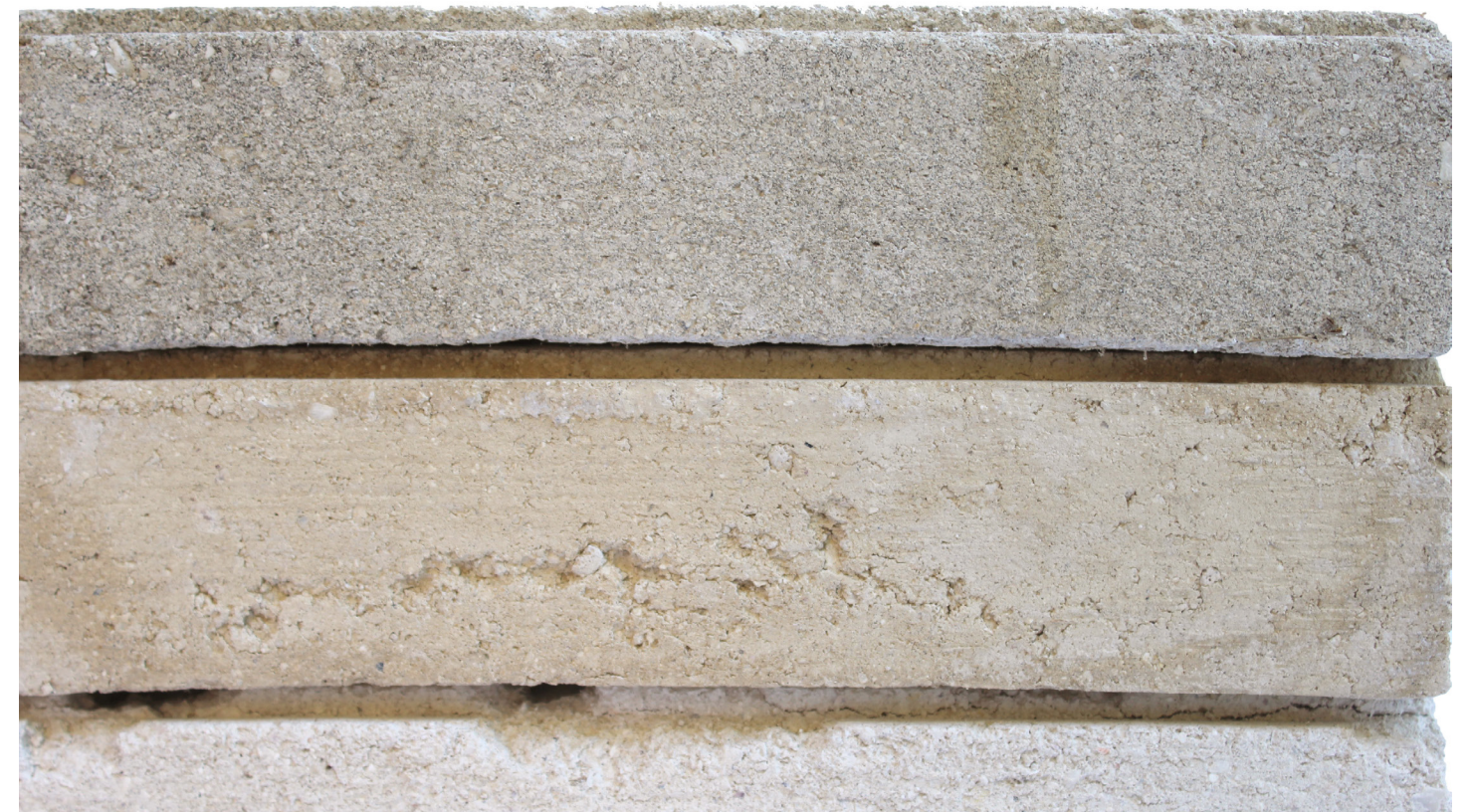
Figure 8.25 The addition of small amounts of rubber powder (top), clay (middle), or no additives (bottom) produced a range of earth tones in the completed bricks. (Photo by Jeremy McGlone)
