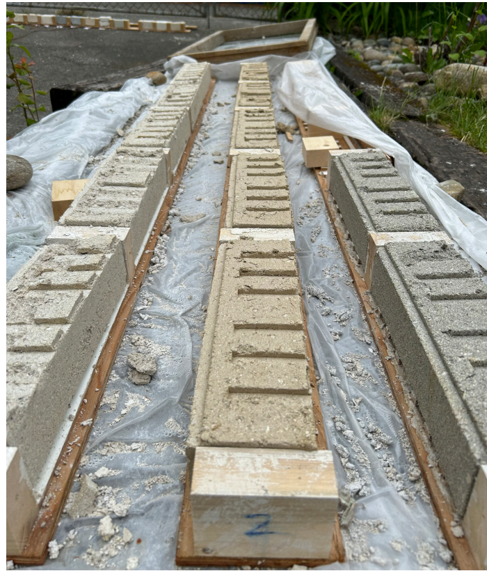
Bricks Rotated and Left to Dry
