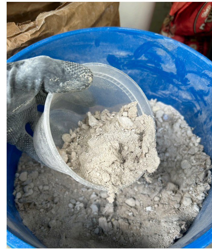
Figure 8.12 Recycled and crushed drywall (Photo by author)
