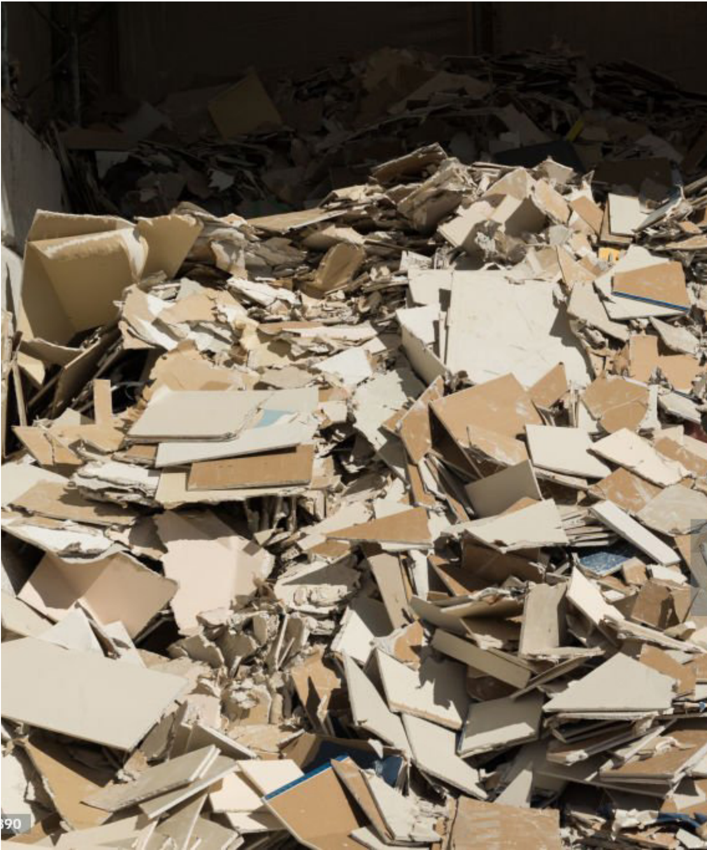
Figure 8.27 As much as 20% of drywall that arrives on site is discarded to landfills as off-cut material (Photo courtesy of AscentXMedia)
