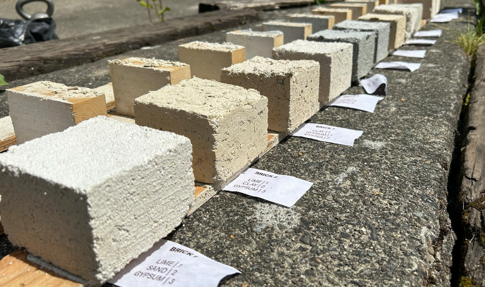
Figure 8.1 An array of sample mixtures testing which ratios of repurposed construction and industrial waste produce the best brick alternative to raw fired clay (Photo by author)
