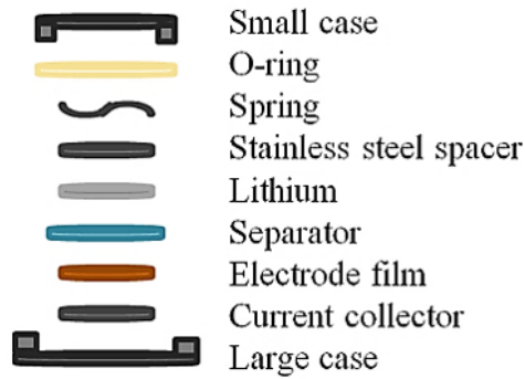
Figure 1-5. Diagram of a typical coin cell.
