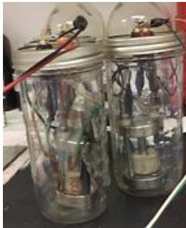
Figure 1-7. Photograph of an assembled cell for ASSB testing. The jar with the binding posts prevents moisture exposure, while the SS parts inside are to provide the ASSB with pressure.
