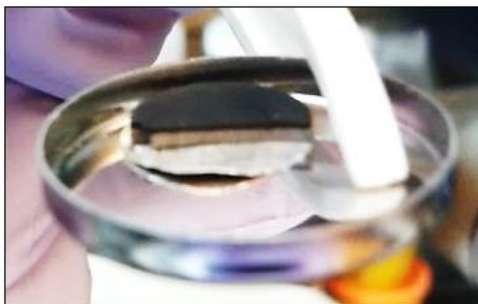
Figure 2-12. Cross section of an ASSB pellet on a 2032 coin cell casing for size reference.
