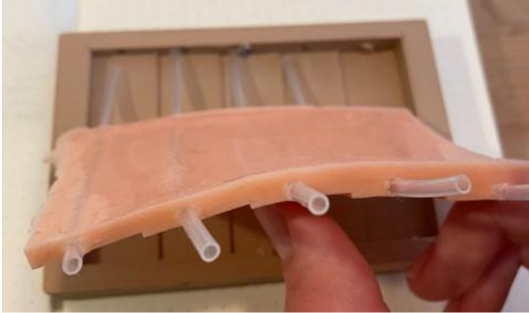
Fig. 33. Variable skin thickness prototype. A silicone skin model with embedded tubing and varying thickness regions (1–5 mm) used to evaluate needle insertion force and optimize tactile realism during venipuncture.
