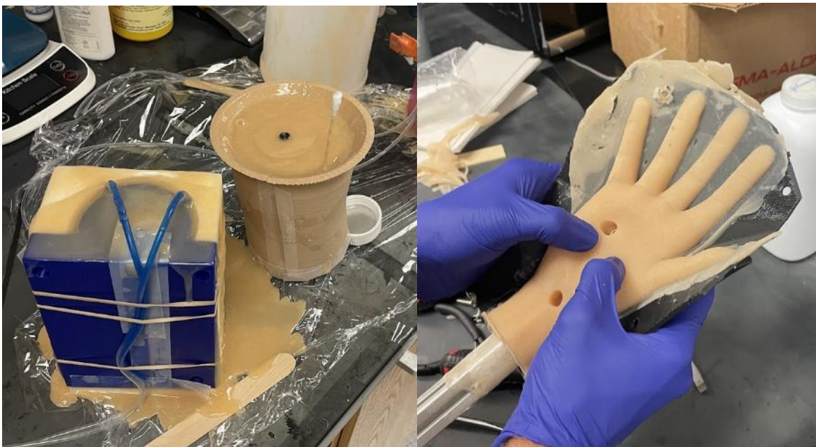
Fig. 32. Early Silicone mold prototypes (a) pour funnels integrated in mold (b) demolding of hand
