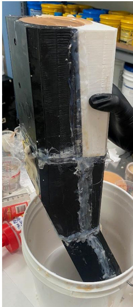
Fig. 23. Hot glue used to seal seams of mold segments
