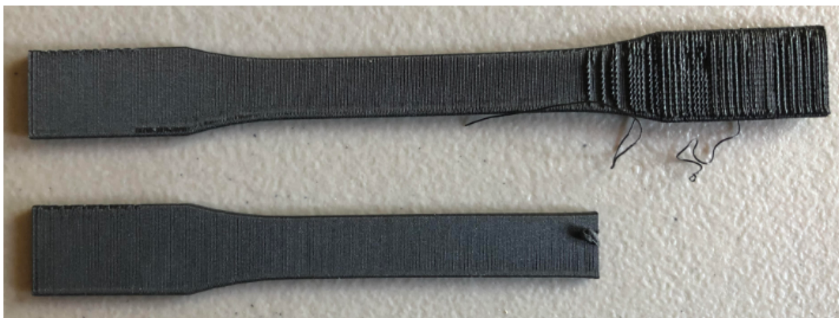
FIGURE 3.5: Typical failed vertical prints with Onyx
