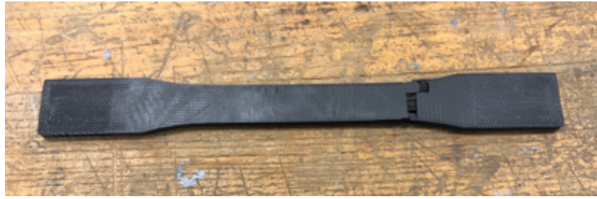
FIGURE 2.20: Onyx with continuous carbon fiber coupon after test
