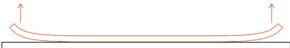
FIGURE 2.8: Warping of 3D printed part [Varotsis, Alkaios B., 2021a]
