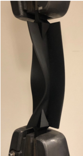
FIGURE 6.3: First T-beam buckled shape at end of test
