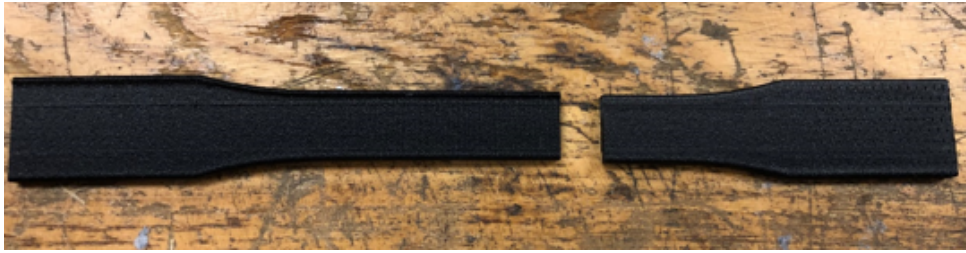
FIGURE 3.19: Vertically printed standard broken coupon
