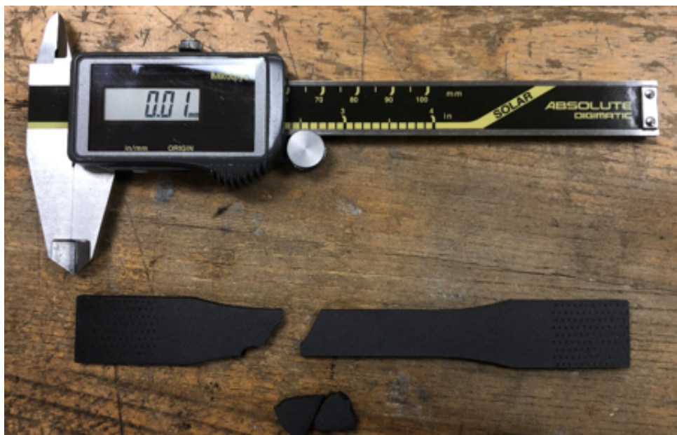
FIGURE 2.13: HT-23 broken tension coupon
