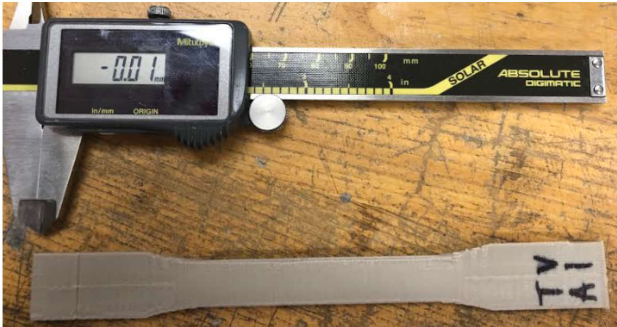
FIGURE 3.8: Successful ThermaX PEEK vertical print
