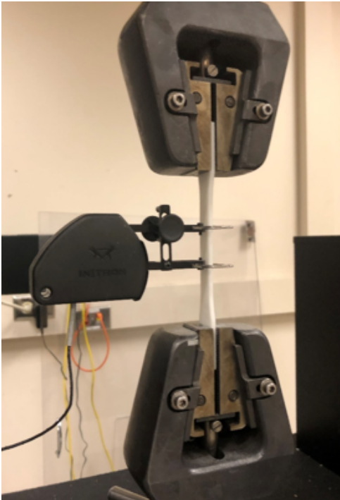
FIGURE A.2: FR-106 Type I tension coupon test setup
