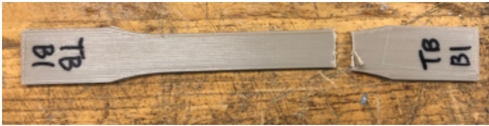
FIGURE 3.9: Type I ThermaX PEEK coupon broken in the radius
