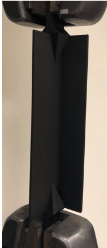
FIGURE 6.1: T-beam before test
