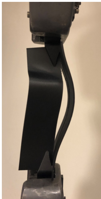
FIGURE 6.5: Second T-beam buckled shape at end of test
