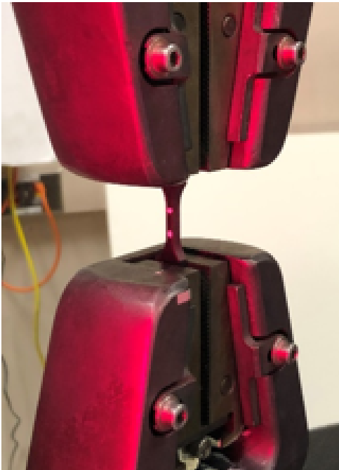
FIGURE A.3: Onyx Type V tension coupon test setup
