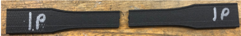
FIGURE 3.20: Vertically printed broken coupon with cold joint broken at the cold joint
