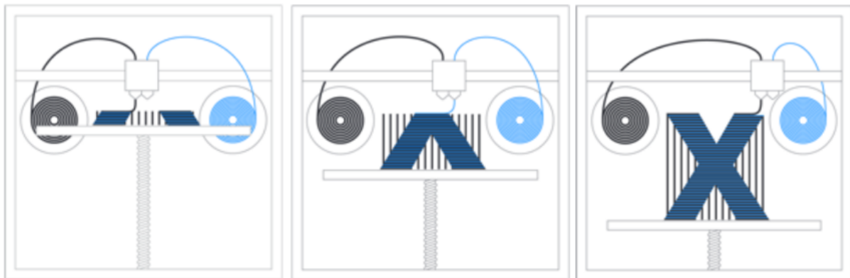
FIGURE 2.3: Printing of an X-shaped part using FFF printing with continuous fiber reinforcing. The print bed is lowered as the nozzles work together to deposit matrix and reinforcing material layer by layer [Markforged, 2021a]
