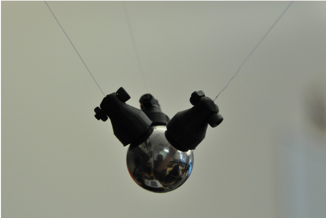
Figure 4.28: Photograph of the final point-mass payload attachment scheme for n = 3 agents. We can note that the tension vector is slightly skewed from acting through the center of mass of the payload, as friction prevents the magnetic anchor from sliding into the ideal placement.
