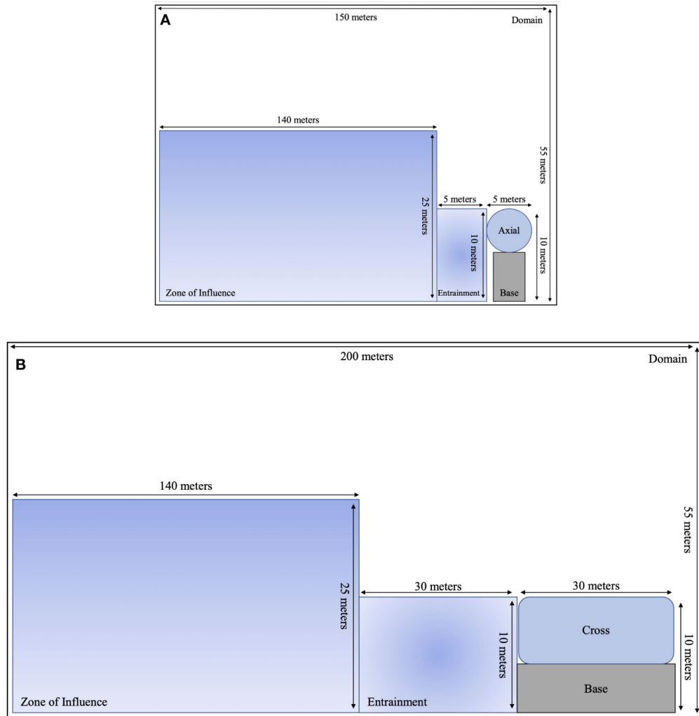
Figure 2. A two-dimensional schematic showing dimensions of the encounter-impact model components for (A) axial and (B) cross-flow turbines.
