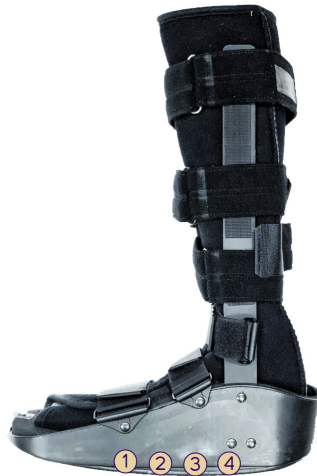
Figure 3.4: The stiff medical boot worn by the participants to minimize ankle flexion and plantar surface forces sensation. Positions of the FSR on the sensor insole at the bottom of the boot are marked accordingly.
