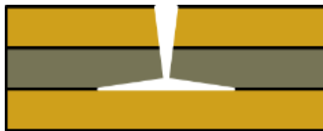
Figure 1. Crack redirection in a nanolaminated metallic system
