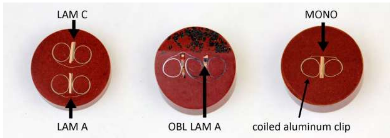
Figure 20. Orientations of the electrodeposited sample beams mounted in bakelite pucks
