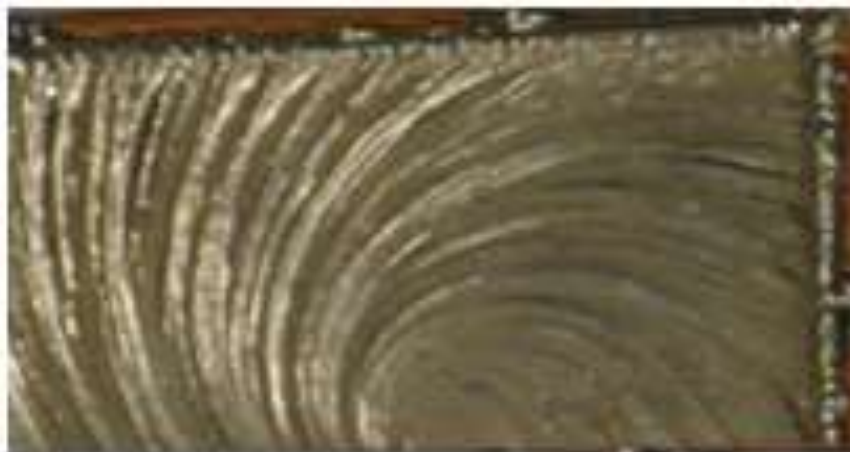
Figure 24. Macroscopic swirls in coating of nanolaminate deposit
