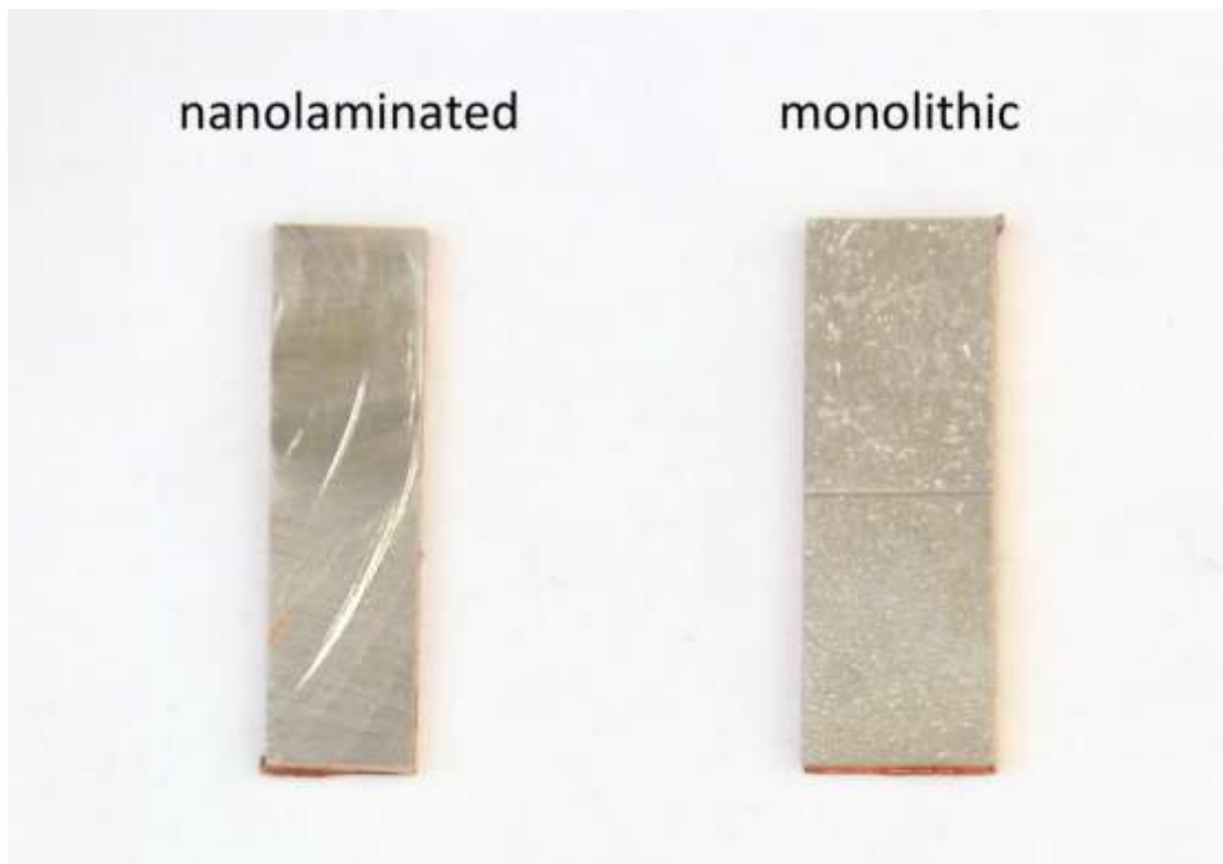
Figure 18. Nanolaminated and monolithic X-ray diffraction samples
