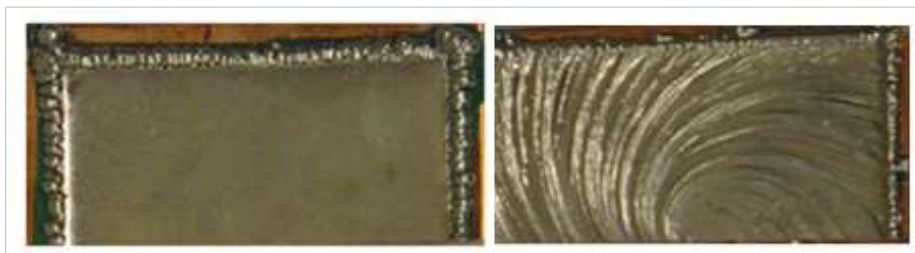
Figure 16. As-deposited coating surfaces from rotating disk electrode samples ( left: monolithic nickel; right: nanolaminate )
