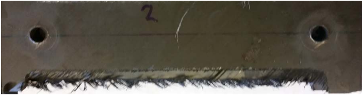
Figure 4-2: Uni Directional composite sample after edge trim (Plan View)
