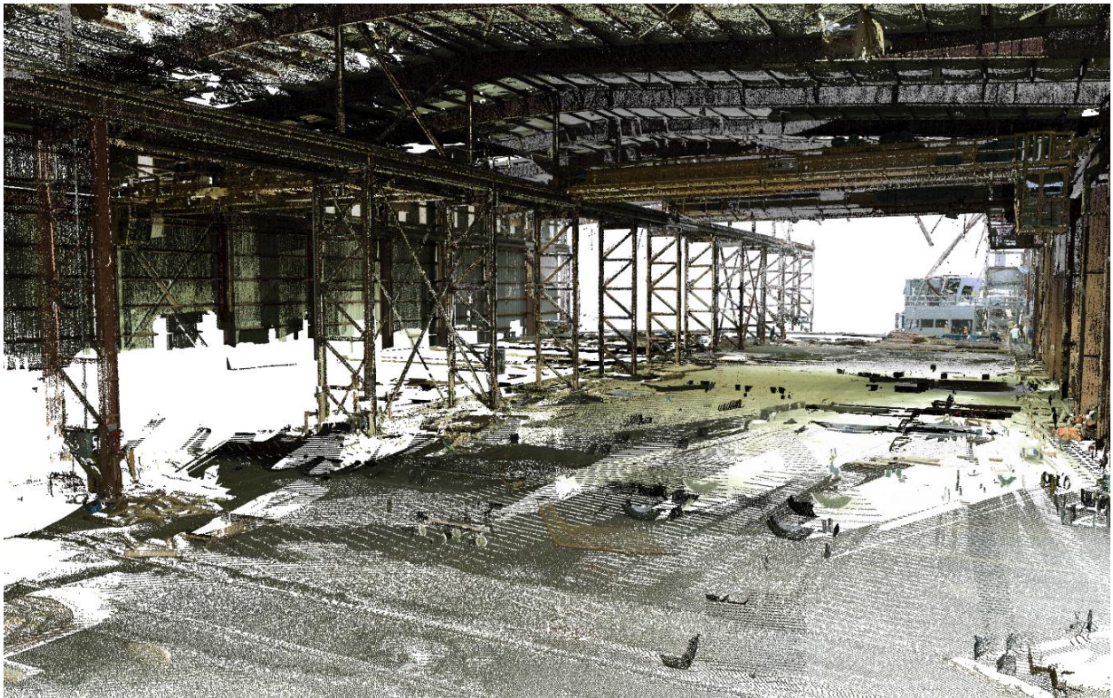
Figure 4.42. Inside view after cleaning showing only XR3 data.
