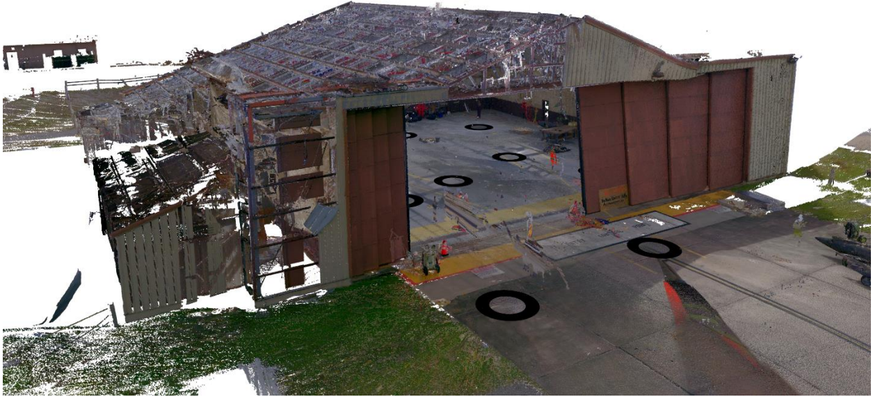
Figure 4.65. Outside view before cleaning showing BLK360 data.
