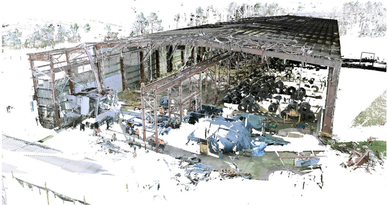
Figure 4.45. Outside view before cleaning showing both BLK360 and XR3 data.
