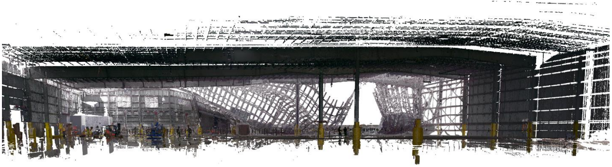
Figure 4.3. Inside view before cleaning showing only BLK360 data.
