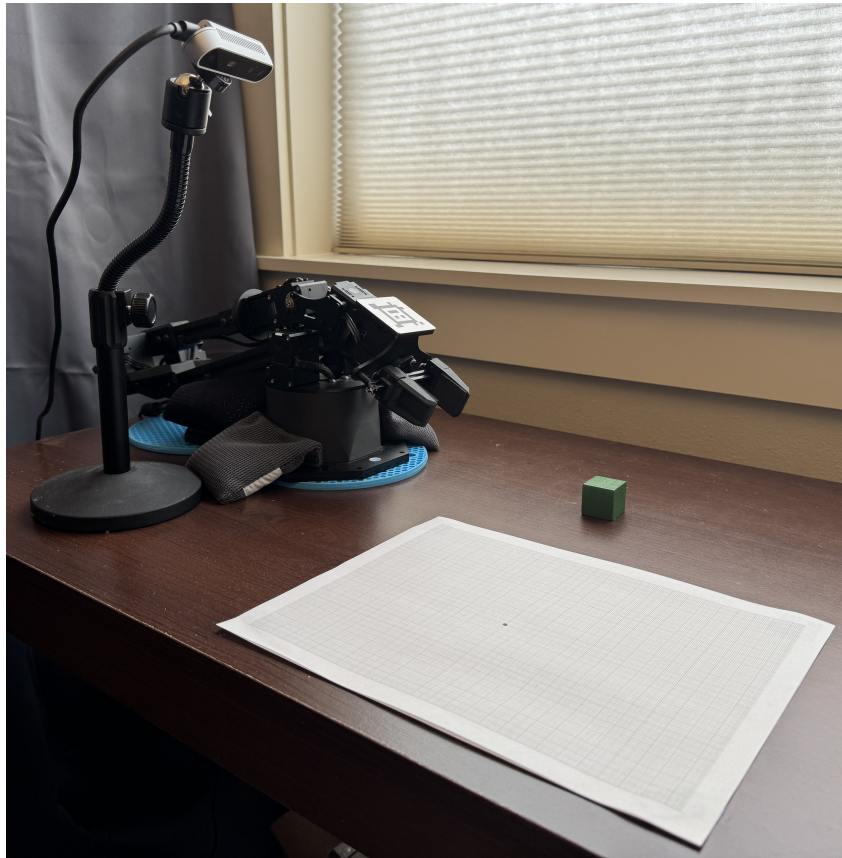
Figure 4.6: VLA-Based Pick and Place Setup (required for inference).
