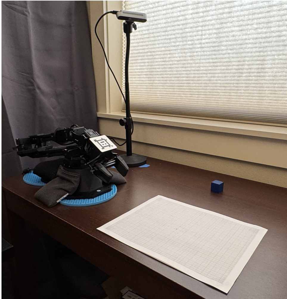
Figure 4.1: Deterministic Pick and Place Setup (required for point cloud rendering).
