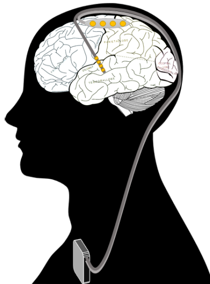
Figure 2.1: An illustration of the Activa PC+S system, incorporating the IPG in the upper chest with wired connections to the ECoG strip over M1 and DBS probe in the thalamus. The IPG is equipped with data streaming and limited data storage capacity.
