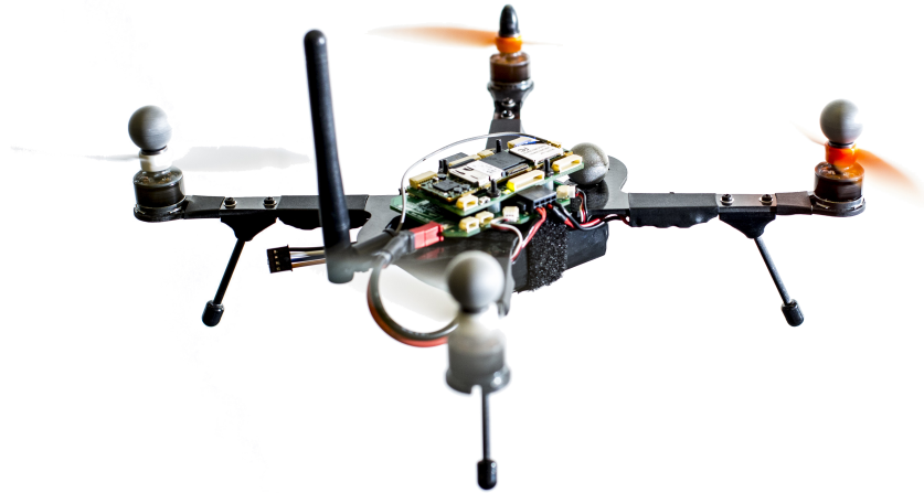
Figure 3.2: ACL’s custom quad-rotor platform. The vehicle is approximately 240 mm long from motor to motor and can hover for over 20 minutes.
