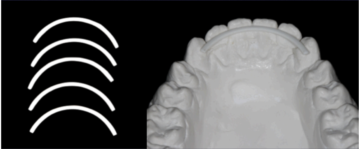
Figure 1. Five exploratory curved Y-TZP specimens with dimensions 1.0 x 0.9 x 36.0 mm and pictured on actual patient model
