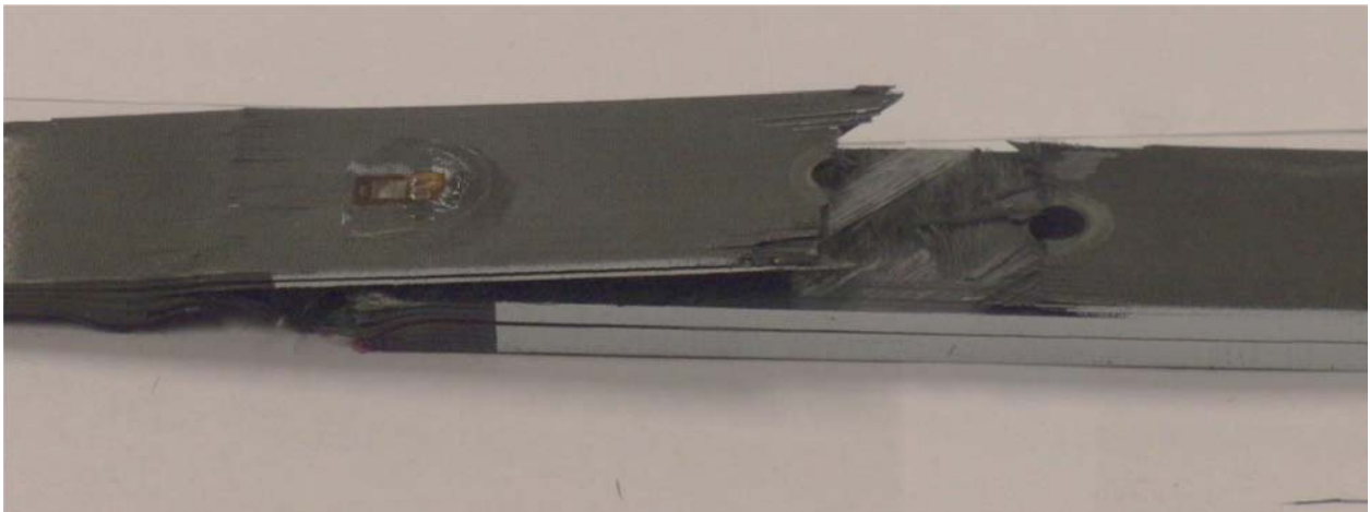
Figure 41. Specimen Ultimate Failure – Filled-Hole Tension Mixed with Laminate Delamination/Splitting
