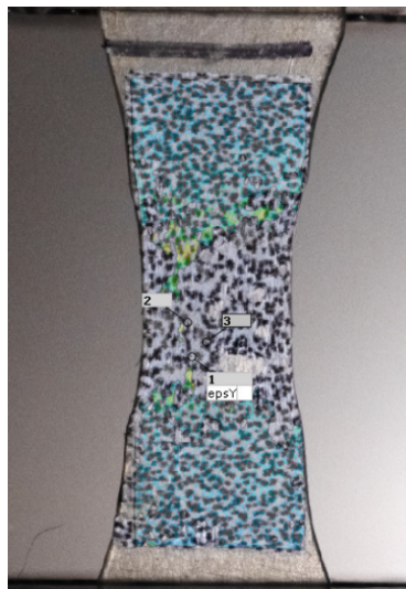
Fig. 32 DIC picture of deformed nanofoam under uniaxial strain on y direction at 390s in the test with marked deformation in x and y direction.
