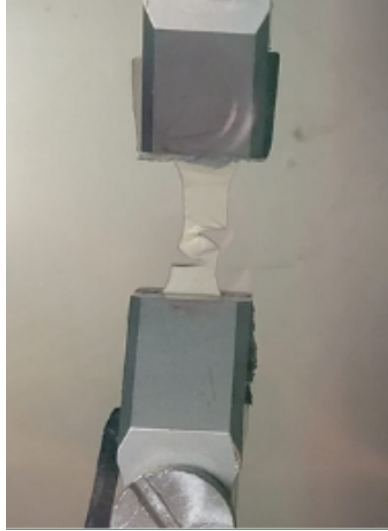
(a) Necking Discovered in DMA.
