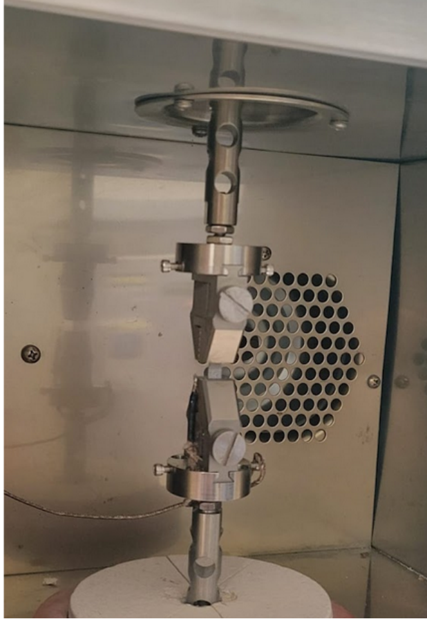
Fig. 22 Tensile Test with Temperature Gradient.
