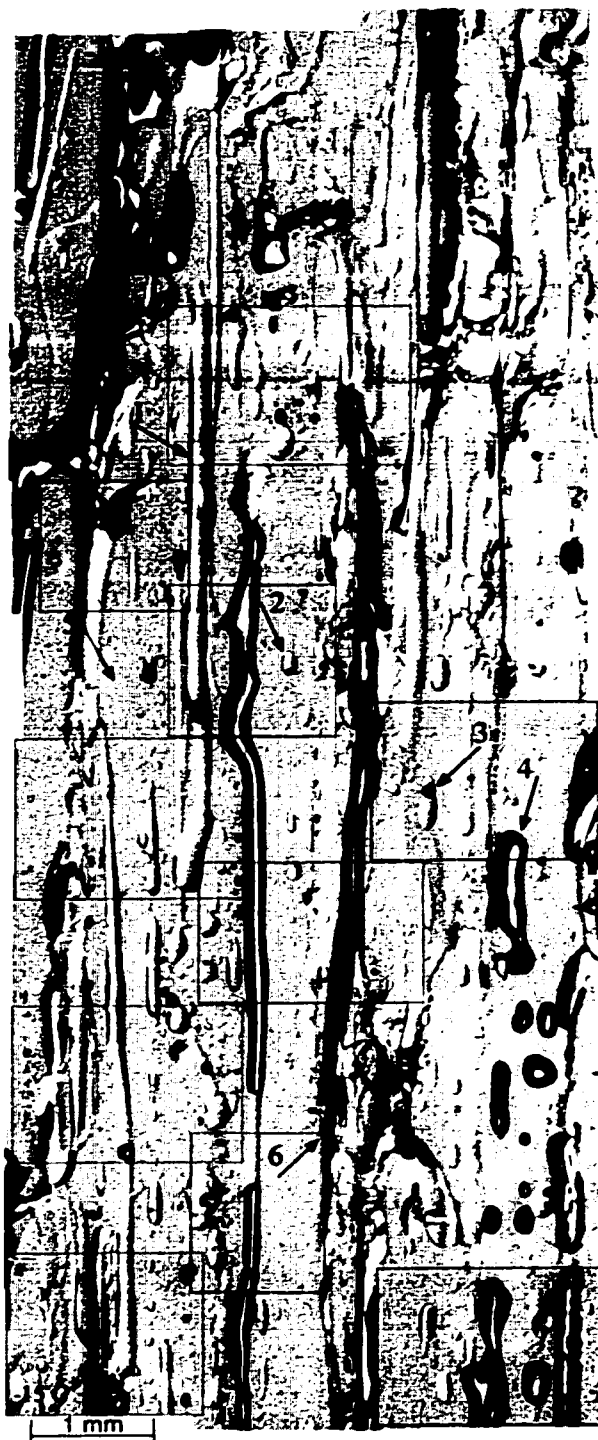
Figure 4.3. Photomosaic of vertical thin section of first-year ice in transmitted light. Ten boxed regions refer to subregions shown in Fig. 4.4. Overall dimensions of scene are approximately 12.1 x 4.7 mm, and the magnification is 15. Arrows indicate examples of (1) brine tubes, (2) brine pockets, (3) vapor bubbles, (4) drained inclusions, (5) transparent areas, and (6) poorly-defined inclusions.
