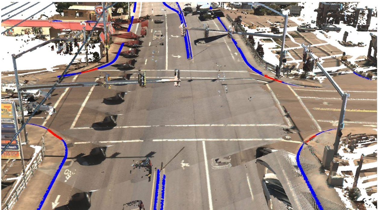
(a) An intersection where all four curb ramps are correctly identified.
