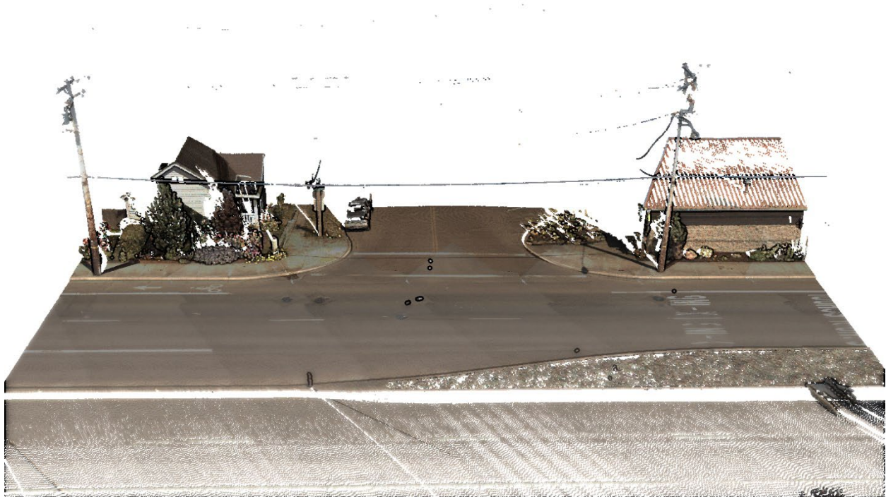
Figure 3-3. The original mobile lidar data.
