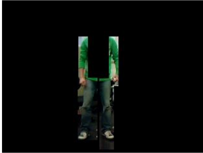
Figure 3.5: An example of four targets for mean shift tracking, including right/left arm, and right/left leg.
