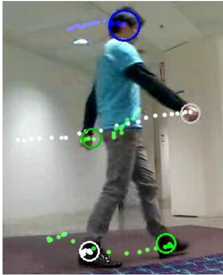
Figure 3.20: The trajectories of the 5 body part blobs, including head, right/left hand, and right/left foot.
