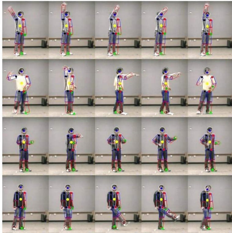
Figure 3.32: The snapshots of the 3D pose estimation results on SR3 videos. From top row to the bottom row, they are waving, throwing, boxing and kicking by four actors.
