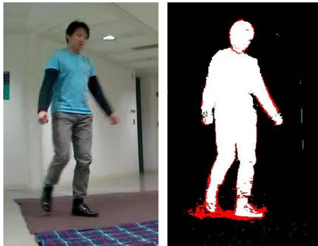
Figure 3.14: The left image is original frame. The right image is the classified frame as four categories, F (white), B (black), S (red), H (green).
