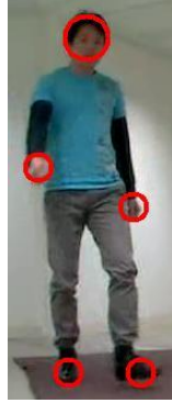
Figure 3.19: The target models of the color of 5 blobs are shown in red circles.
