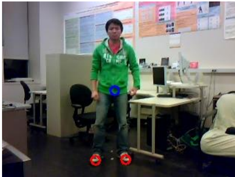
Figure 3.4: Feet identification. The blue circle is the reference point, and red circles are detected feet blobs.
