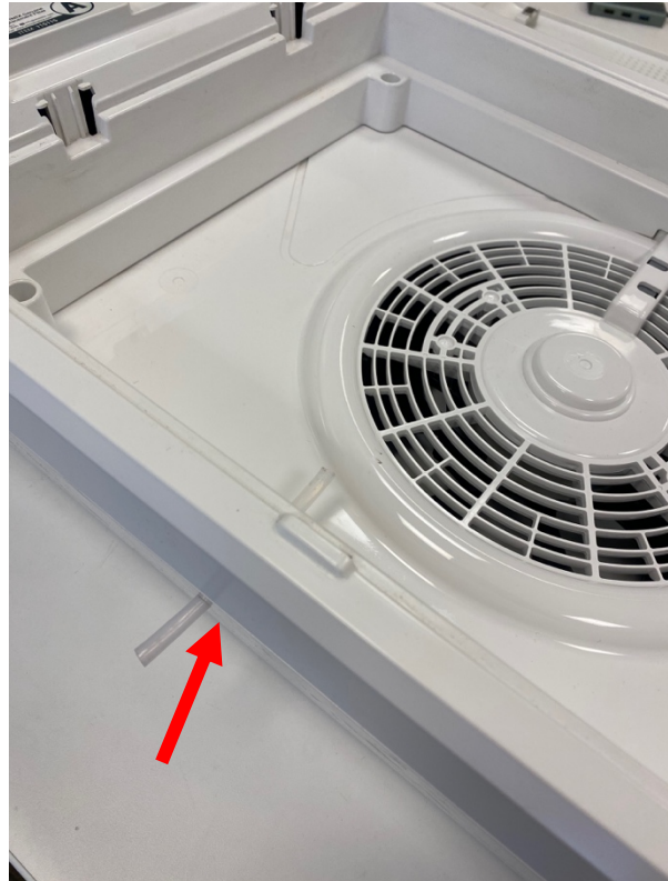
Figure 1. Photos of the (a) custom-built plywood chamber and (b) the location of the pressure sensing tube on the PAC body.
