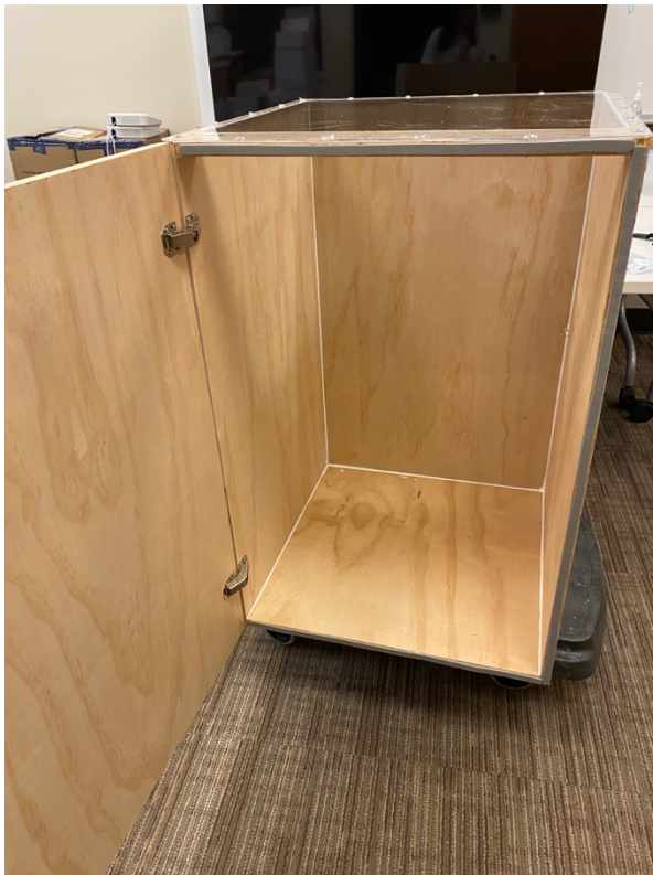
Figure 1. Photos of the (a) custom-built plywood chamber and (b) the location of the pressure sensing tube on the PAC body.
