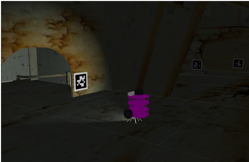
Figure 4.12: Example picture of the Gazebo simulation with the purple TurtleBot3 Burger running in the ballast tank in Fig. 4.2, with rusty texture and no external light source. A few scattered AprilTags are used as known features in the tank.
