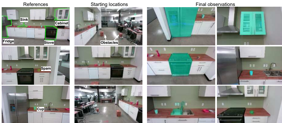
Figure 4.11: Real kitchen experiments. Left: reference images and contours of target object masks. While the fridge is partially out of view, the model can still reach the fridge. Middle: Initial view of the scene through the tilt camera. Right: robot observations after reaching each object overlaid with predicted masks (in cyan).
