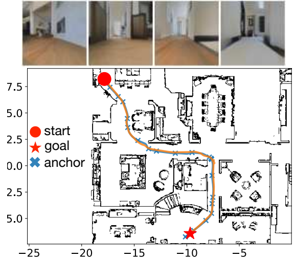
Figure 2.6: Following a 23m long trajectory. Blue trace: groundtruth trajectory. Orange trace is generated by following the anchor points.
