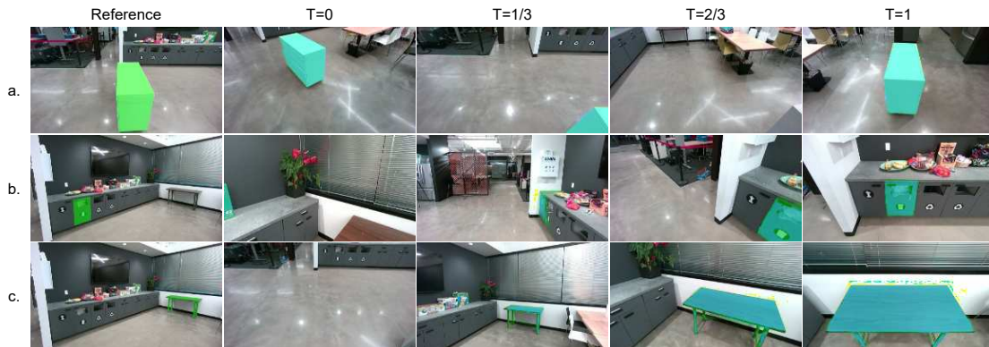
Figure 4.12: Real-world qualitative experiments in new scenes. Left: reference image with target object highlighted by the green mask. Remaining columns: robot's camera view at T = \{0, 1/3, 2/3, 1\} . The tracked object is highlighted by the cyan mask. The tasks are: (a) Go to the back of the cabinet and stand 0.8m away. (b) Go to the front of the landfill trashcan and stand 1m away. (c) Go to the front of the table and stand 0.5m away.
