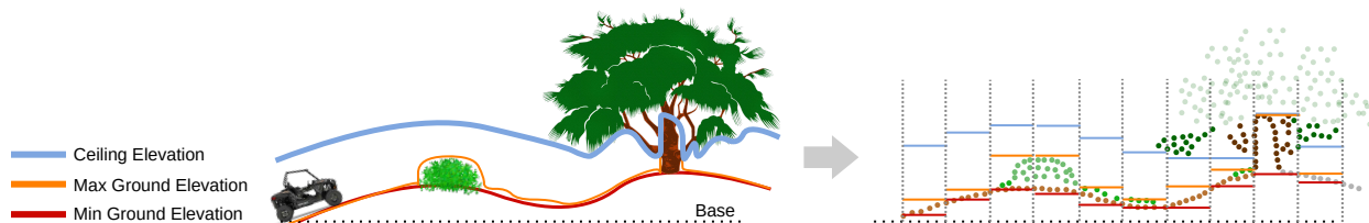
Figure 3.7: Left Multi-layer terrain representation. The ground layer consists of the minimum and maximum ground elevations to capture the sizes of porous objects like bushes and also preserve sharp elevation changes after discretization. The ceiling layer represents the geometry of the overhanging objects (e.g., canopy) that might potentially block the path. Right In our practical implementation, we obtain a dense point cloud of the environment, discretize the x - y plane into 2D grid cells (shown in 1D for simpler visualization), and compute the elevation values by analyzing the point distribution in each cell. We ignore anything higher than the desired vertical clearance. For each layer and each cell, we count the number of semantic points for each class and compute a normalized histogram as the semantics of that cell.
