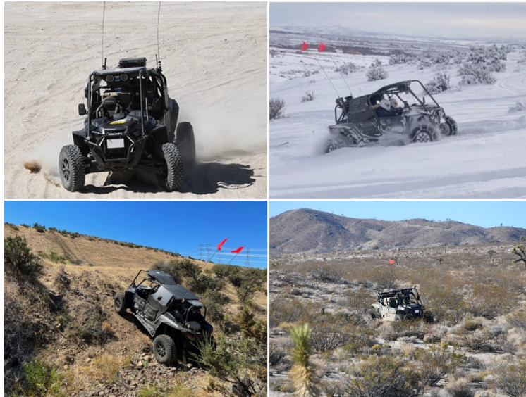
Figure 3.6: High-speed driving in complex off-road environments requires joint reasoning of terrain semantics and geometry. Top row: a vehicle can drive at high-speed on a dirt road but has to be more cautious in snow due to wheel slipping. Bottom row: a vehicle needs to estimate terrain slopes and sizes of vegetation for safe planning and control.
