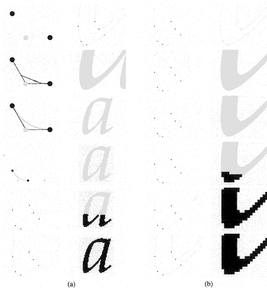
Figure 4.4 Using animation to expand and compress detail. The figure has three levels of detail: a closeup on the three points defining one curve segment, and intermediate level showing curves connecting end-to-end, and an overall view showing the whole character as it is filled with pixels. In part (a), animated zooming is used to smoothly connect the three levels, so each can be shown full-screen. In part (b), the animated content is the same; only the zoom is missing. Now the screen is too cramped for the final part of the sequence, while it is hard to see the detail of the initial part.
