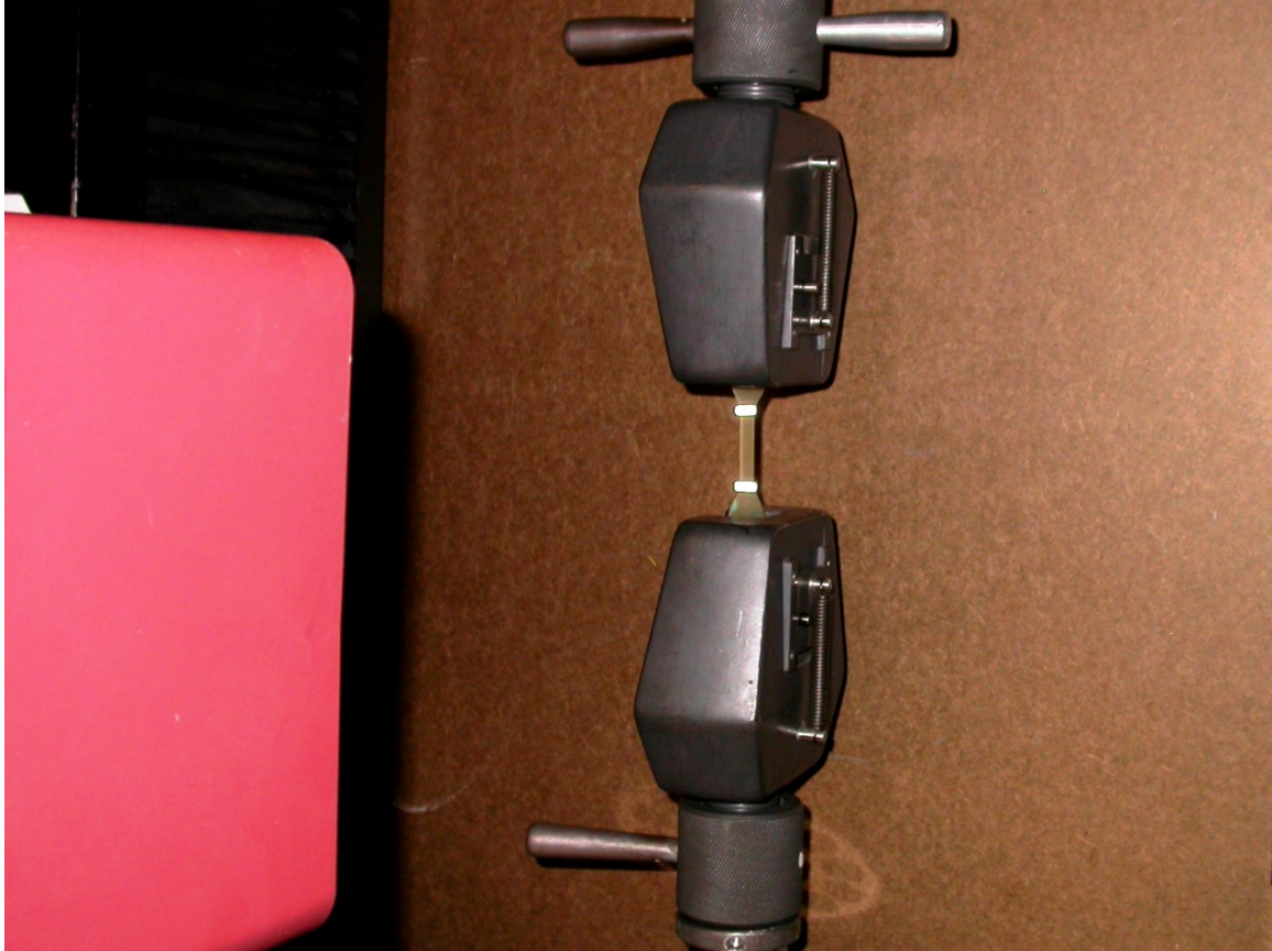
Figure 54: Tension test setup showing laser extensometer targets on IPN tension specimen (laser extensometer on left)
