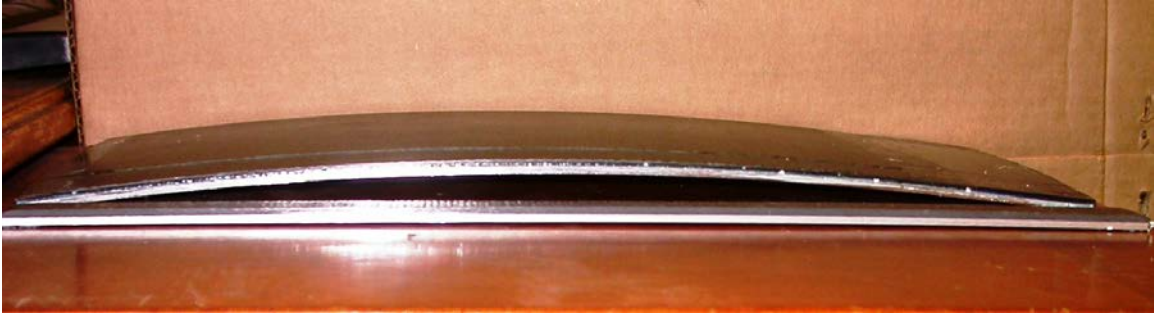
Figure 47: Relative distortion of IPN adhesive (front) and film adhesive (rear) specimens
