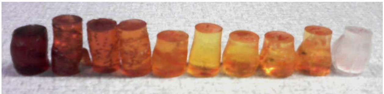
Figure 75: UV-cured compression test specimens in the BPADA + (50-50)Epoxy material system (after testing)
