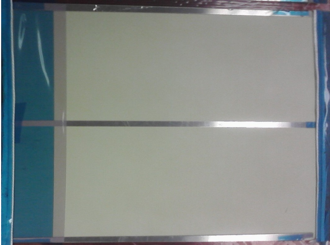
Figure 46: Aluminum adherend with shims prior to bonding with IPN adhesive
