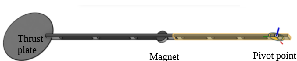
Figure 4-1 Pendulum modeled using Onshape (90 degree rotation)
