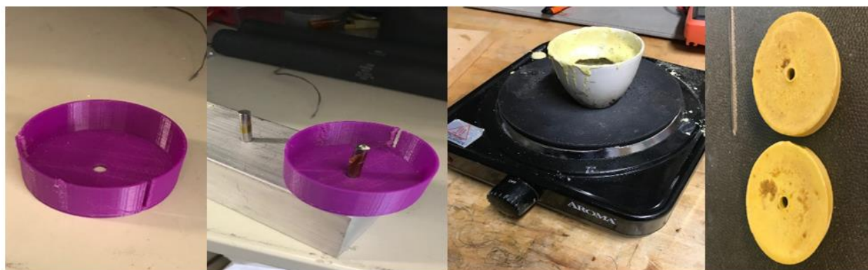
Figure 4-3 Sulfur puck formation with 3D printed PETG molds, tungsten center rod with aluminum heat sink, hot plate heating, and final pucks shown
