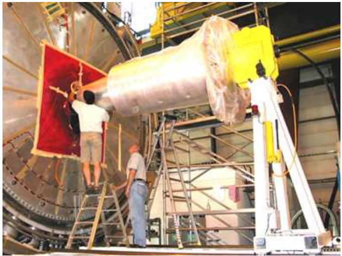
Figure 3.18: Left: Schematic detail of tube structure for the hadronic FCal modules, showing the tungsten slugs surrounding each tube. Right: Completed FCal assembly being inserted into one of the endcap cryostats.
