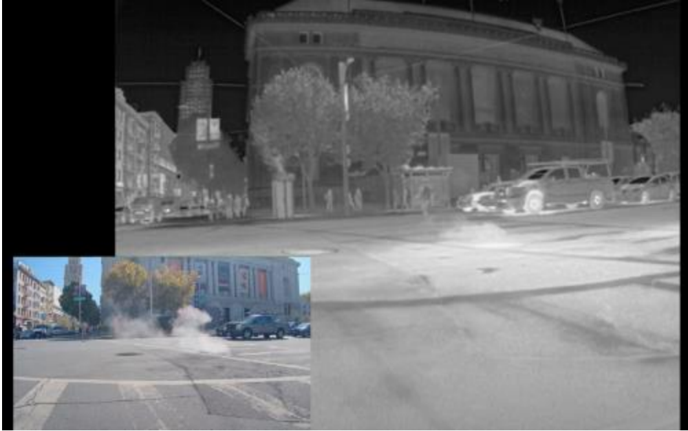
Figure 5: A pedestrian is completely obscured by smoke during daytime. A FLIR camera is still able to detect them. Rangwala, Sabbir. “Thermal Cameras Gain Acceptance for ADAS and Autonomous Cars.” Forbes
