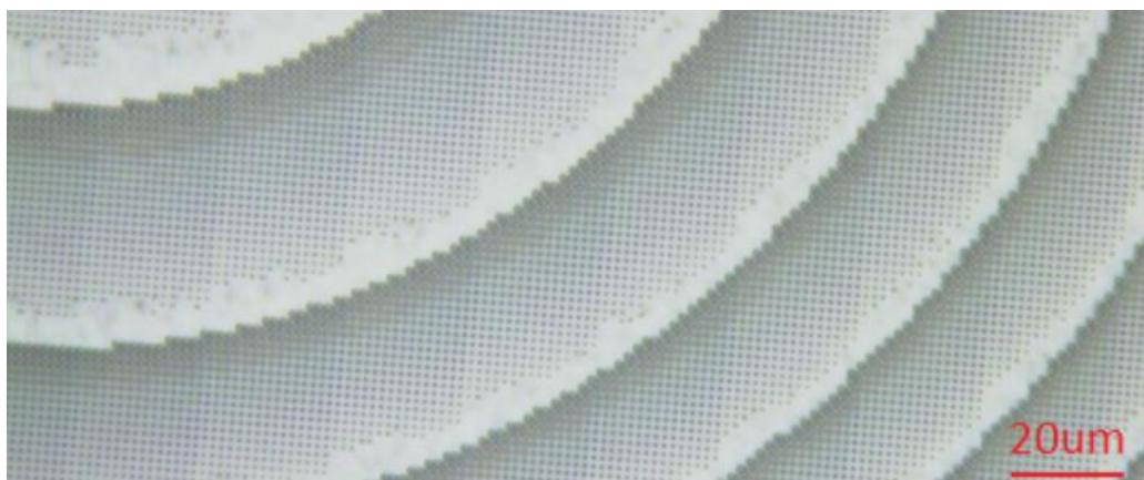
Figure 11: Pillars collapsing issue
