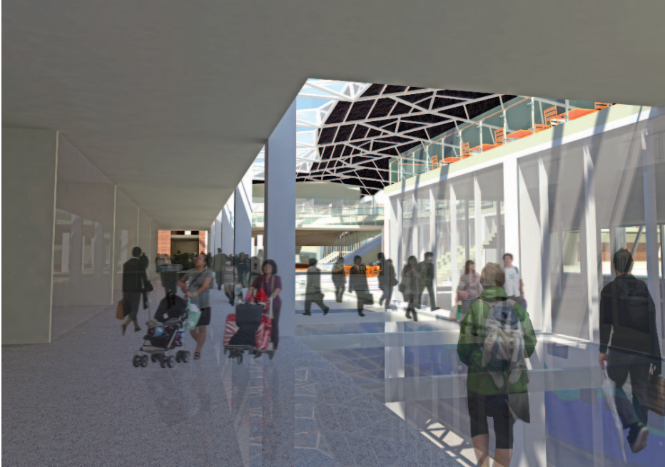
Figure 7.17 - View 2 of the internal pedestrian corridor with glazed floor to allow for natural light to platforms. Views to trains constant reminder of trains below.
