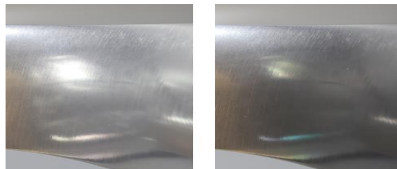
Figure 2.8: Using polarizing filters – (left) Unpolarized, (right) Polarized
