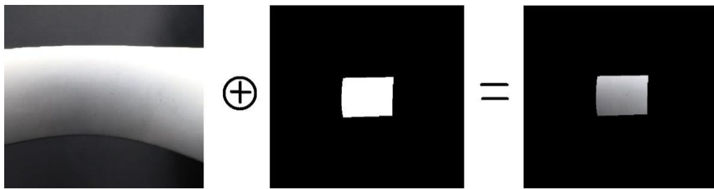
Figure 2.5: Illustration of the bit-masking process – (left) Input, (center) Mask, (right) Output
