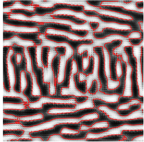
Figure 2.2: A 2D slice of the GRF for the gradient architecture. The red curves represent the position of the isosurface in the structure.
