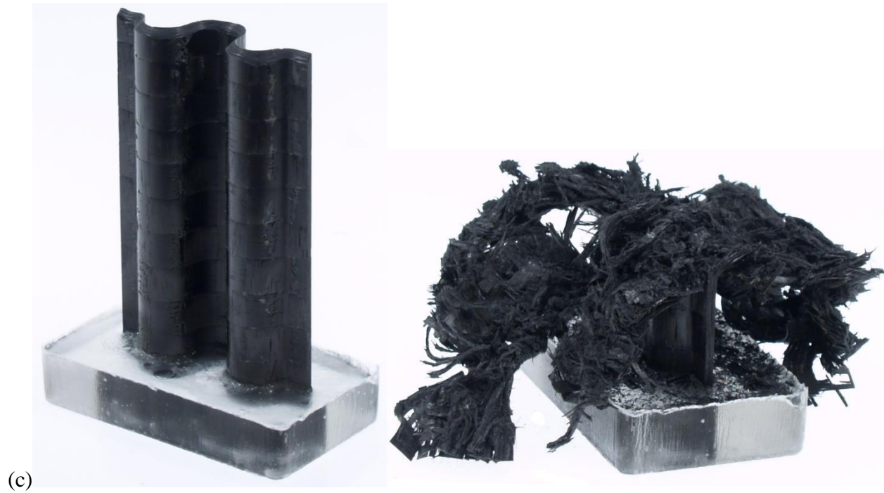
Figure 20. (a) Low sinusoid, (b) high sinusoid, and (c) semi-circular corrugated crush specimens before and after testing.
