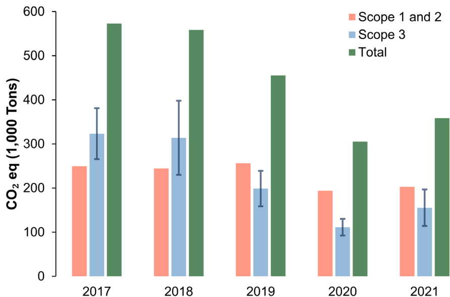
Figure 5.2 Comparison of Scope 1 and 2 greenhouse gas emissions with Scope 3 for WSDOT as an agency from 2017 to 2022. Results suggest a relatively equal share of Scope 3 emissions from roadway construction in total WSDOT greenhouse gas emissions. The error bars in this graph denote standard deviations due to the uncertainty of emission factors used to run LCA on entire projects and HMA line items.
